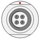
Note\*\*) Both PWR pins 1&2 must be connected! Note\*\*\*) Both GND and pins 3&4 must be connected!
