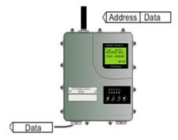
Reception addressing has been set ON and either the primary or secondary RX address of the radio modem is identical to the address of the received data packet.
