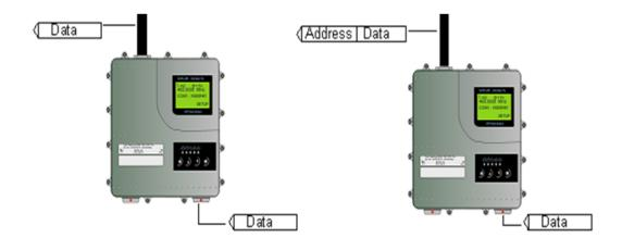
Transmission address has been set OFF. Radio modem will transmit the data packet as such.
